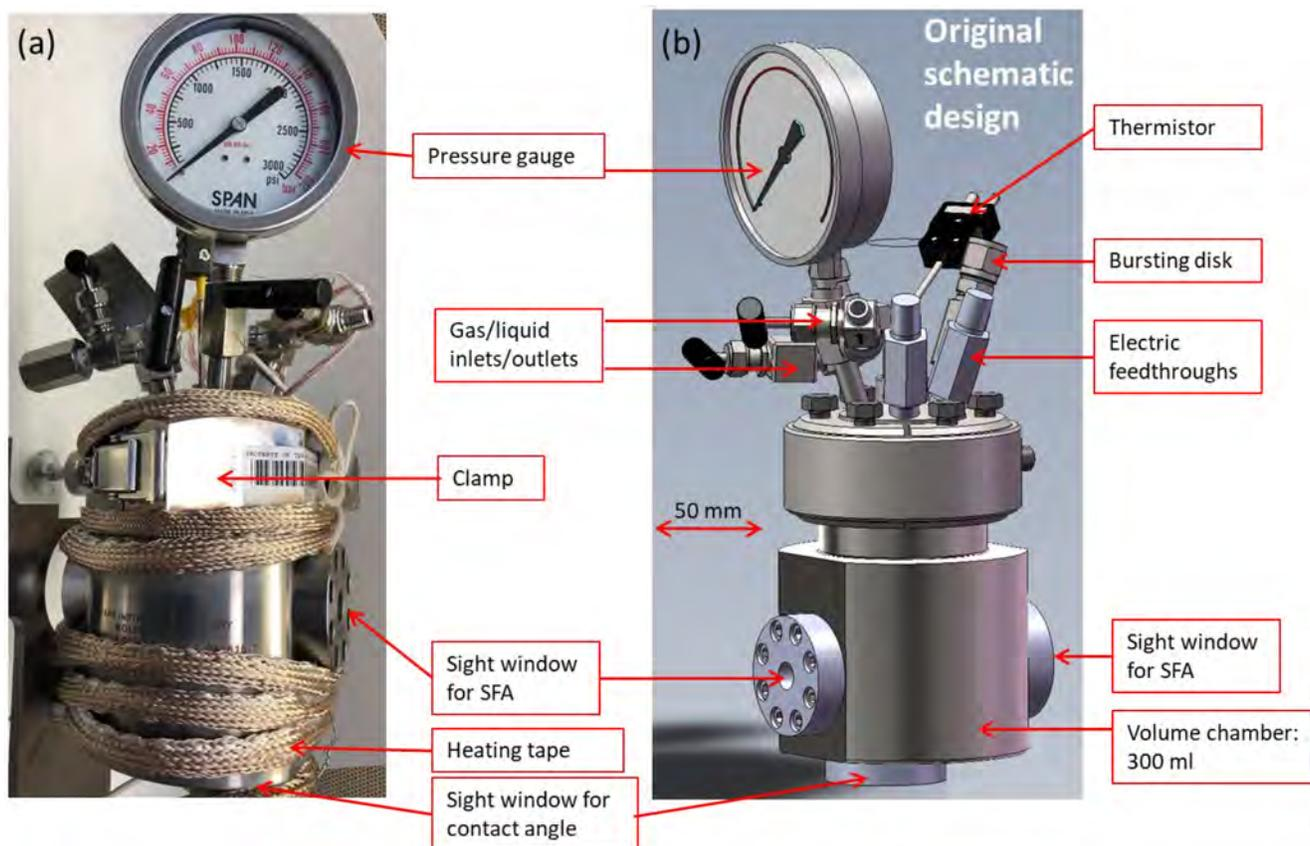
Figure 3—The pressure vessel for the HTHP-SFA. (a) A photo and (b) the schematic of the pressure vessel purchased from Parr Instrument Co. This is certified to withstand 3000 PSI (204 atm) and 225°C. Our new design of the Surface Forces Apparatus and Contact Angle device fits inside this pressure vessel.
