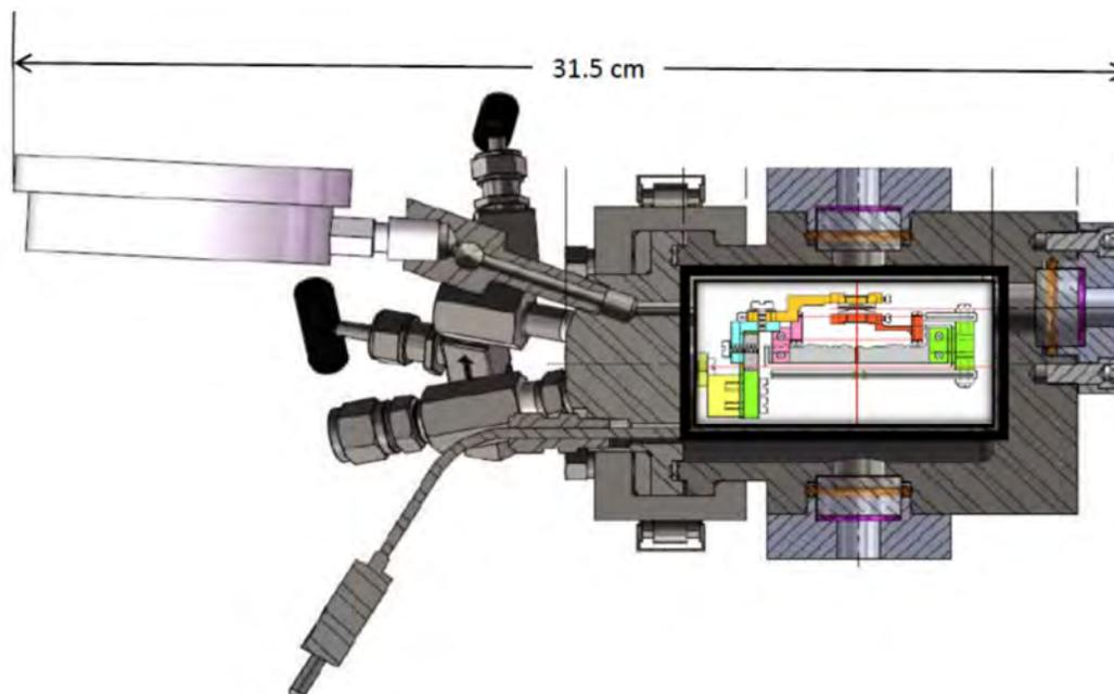
Figure 4—Schematic design of the HTHP-SFA with a custom designed SFA. The custom designed SFA, see details Figure 5, is placed inside a pressure vessel from Parr Instrument.
