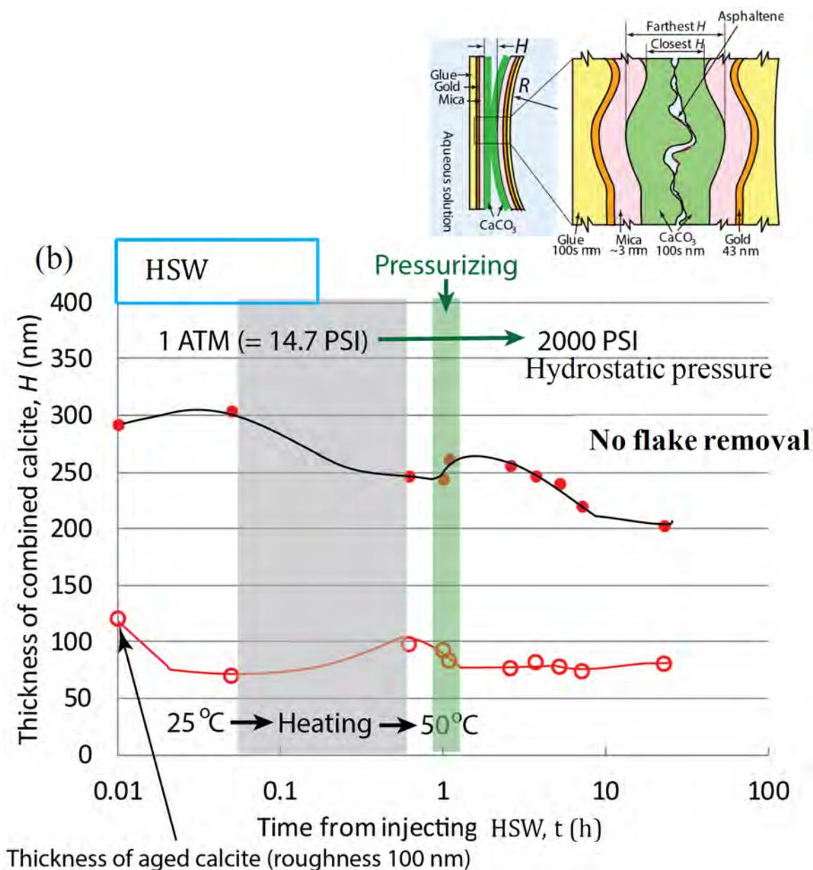
Figure 7—Changes in the maximum and minimum thickness of a pair of calcite surfaces (see inset) as function of time in HSW. After the calcite surfaces were inserted, the SFA chamber was heated up to 50°C. After one hour, the SFA chamber was pressurized from atmospheric pressure to 2000 PSI. HSW does not remove add-layers, resulting in no significant thickness change. The saturation index of calcite in HSW (1 atm, 100°C) is -0.5.
